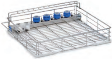
LOAD BASKET WITH 4 WAND HOLDERS, 5 INJECTORS FOR HOLLOW ITEMS AND 2 CONNECTIONS FOR ASPIRATION TUBES.
